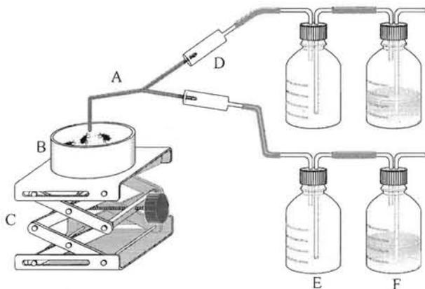
Fig. 1. A schematic diagram of the Y-track olfactometer. A: Y-track, B: weevil release container, C: a lab jack, D: air outlet, E: a wash bottle for the odor samples, F: a wash bottle for humidification.
