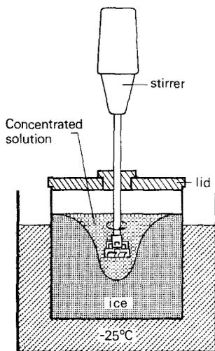
FIG. 2. Freeze concentration arrangement. A stainless-steel jar containing one liter of precooled distillate is inserted in a methanol bath of  $-25^{\circ}\text{C}$ . While the mixture is cooled and stirred, the water is selectively frozen out, leaving the volatiles concentrated into a conical hole.
