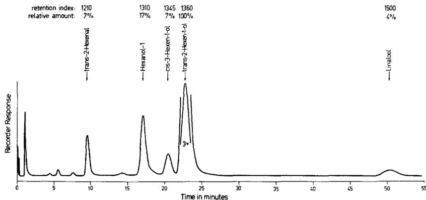
FIG. 3. Gas chromatogram of the potato plant oil: 0.1  $\mu$ l of oil injected on a stainless-steel column, 3 m long and 4.4 mm ID, filled with 10% Carbowax 20M on Chromosorb P-AW-DMCS, 60–80 mesh. Chromatogram run isothermally at 100°C, carrier gas nitrogen at 30 ml/min. Retention indices were calculated according to Kováts (1961).
