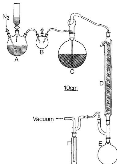
FIG. 1. Vacuum steam distillation apparatus. A: steam generator, filled with 1 liter of bidistilled water; B: steam drier; C: sample flask, containing 2.5 liters of potato plant filtrate; D: condenser; E: receiving flask, set in ice-water bath; F: cold trap, cooled in liquid nitrogen. Preceding the distillation, nitrogen was passed into the steam generator.
